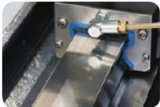
Roller guides on all linear axes for increased rigidity
