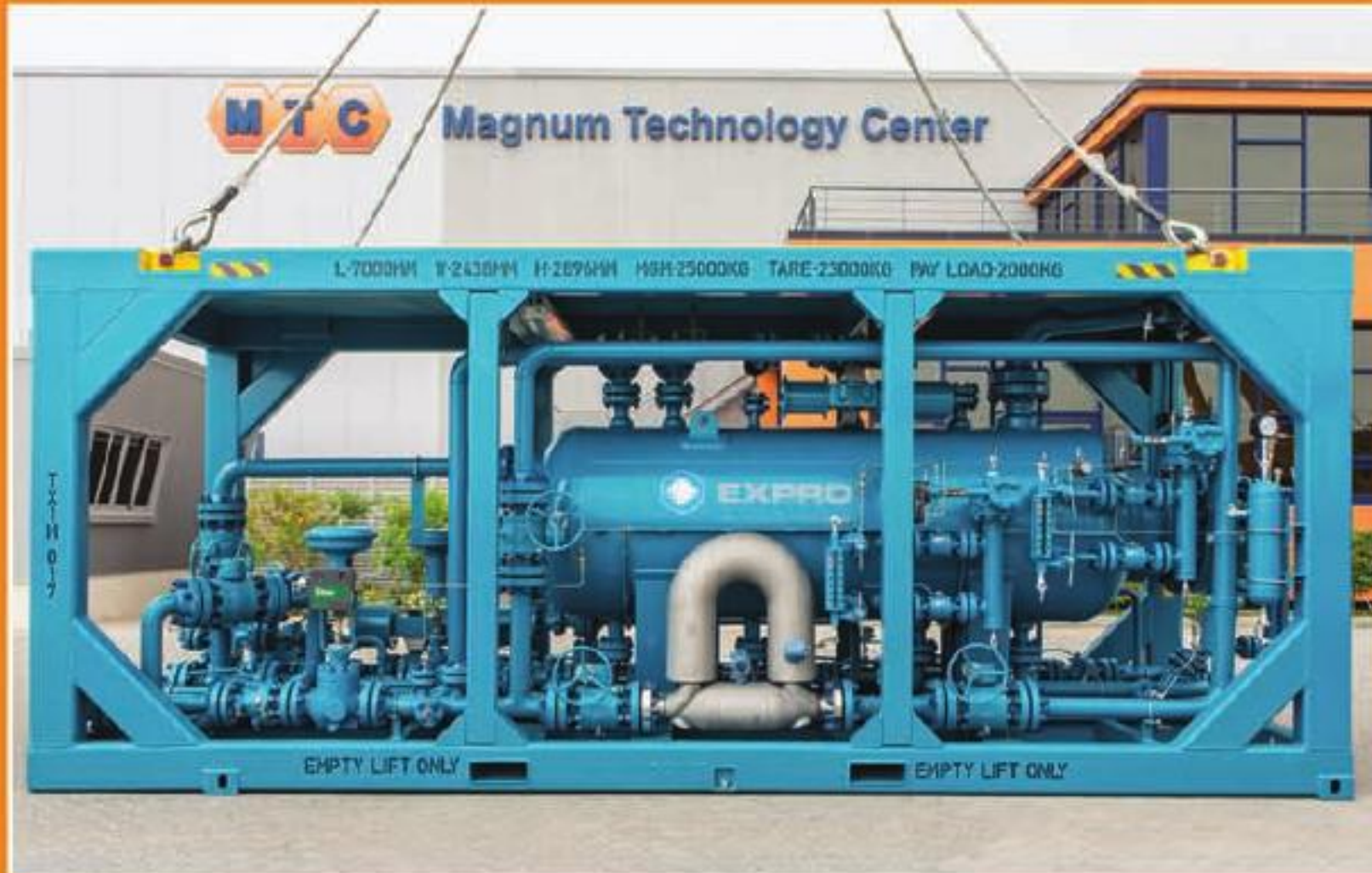
2000 Psi Separator in offshore DNV frame
